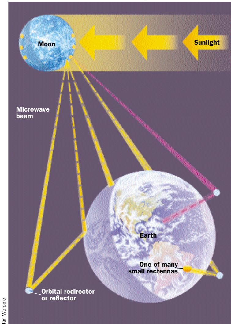
**Figure 2. A “lens” at a base on one side of the moon (or at a linked base on the other side, if sunlight dictates) directs a microwave beam to a relay satellite or directly to a field of rectifying antennas (a rectenna) on Earth.**
